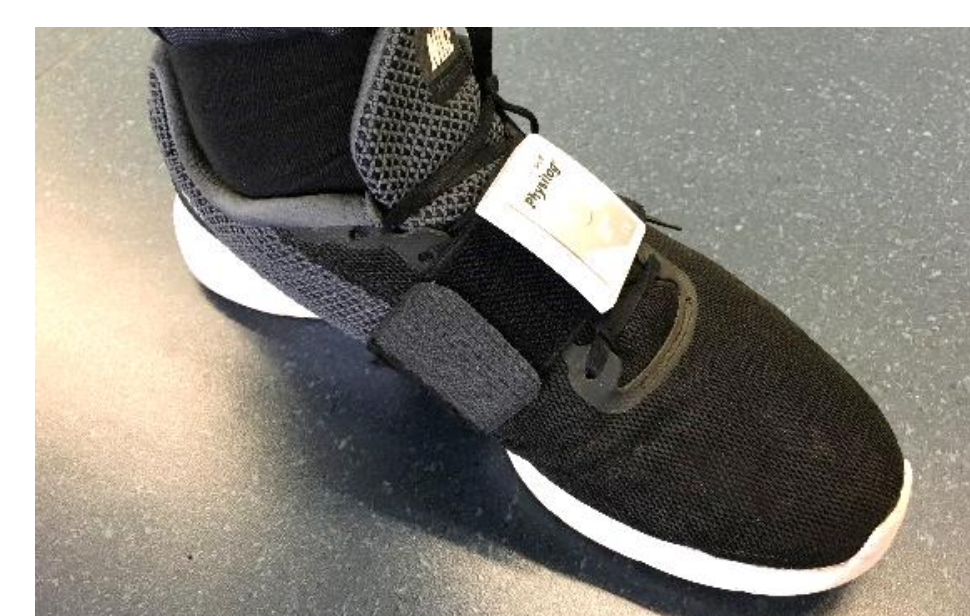
Fig. 1 : foot-worn inertial sensors (Physilog® - GaitUp, Switzerland)
